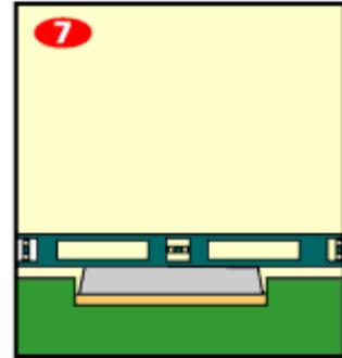
8. Once the stone is level, fill in the area around the stone with soil and tamp it firmly.
