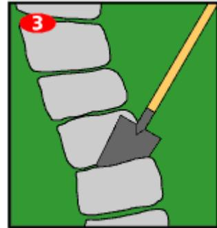
4. Then remove the stone and dig out the sod and earth within the outline so that the stone will sit about an inch above the ground once you have poured an inch of sand into the hole. You will need to consider the thickness of each stone in this step.
