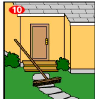
11. Over time you will find that the stones will settle. You can adjust the height or the level of the stones by simply lifting the stone and filling in the hole with some sand or soil.
