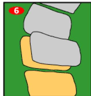
7. Use the level to make sure the stone is relatively level. Push on the stone to make sure it does not rock. You can add or remove sand to accommodate for oddly shaped stones at this point.
